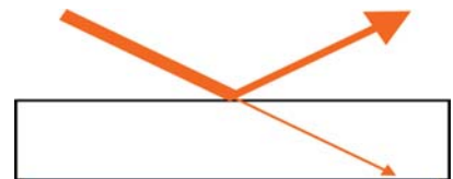
Standard-PV-Module - high reflexion
